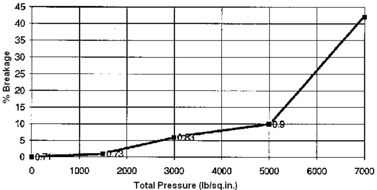
NOTE: The decimal on the curve represents the P-SL50 specific gravity at the corresponding % breakage and total pressure.
